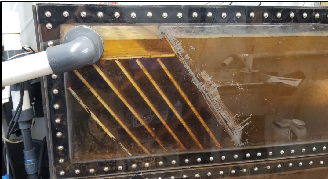
Figure 4: IPS Settling Tank Plates
