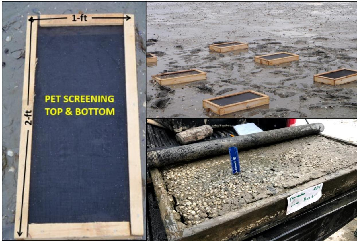
**Figure 3:** Left – recruitment box with Pet screening® (aperture = 1.7 x 0.9 mm); Upper right – deployment of six boxes on a mudflat in the Harraseeket River (Freeport, ME) in a 2 x 3 matrix with 1 m spacing between rows and columns. Lower right – recruitment box (deployed empty in early June 2018 in the St. George River Estuary – Thomaston, ME) that is filled with muddy sediments, and contains 1,875 wild soft-shell clam recruits (shell length range = 1.6 - 22.2 mm).
