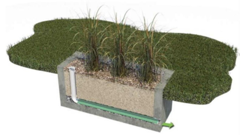
Example of Filterra Stormwater Bioretention System (Image Credit: Contech Engineered Solutions )
